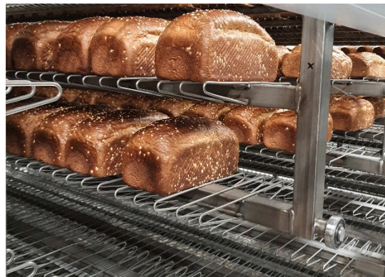
Figure 1. Cooling conveyor hanger with bread
