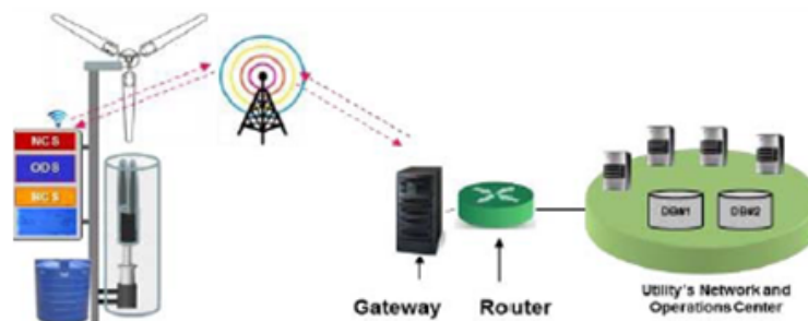
Figure 4. Local network communication subsystem
