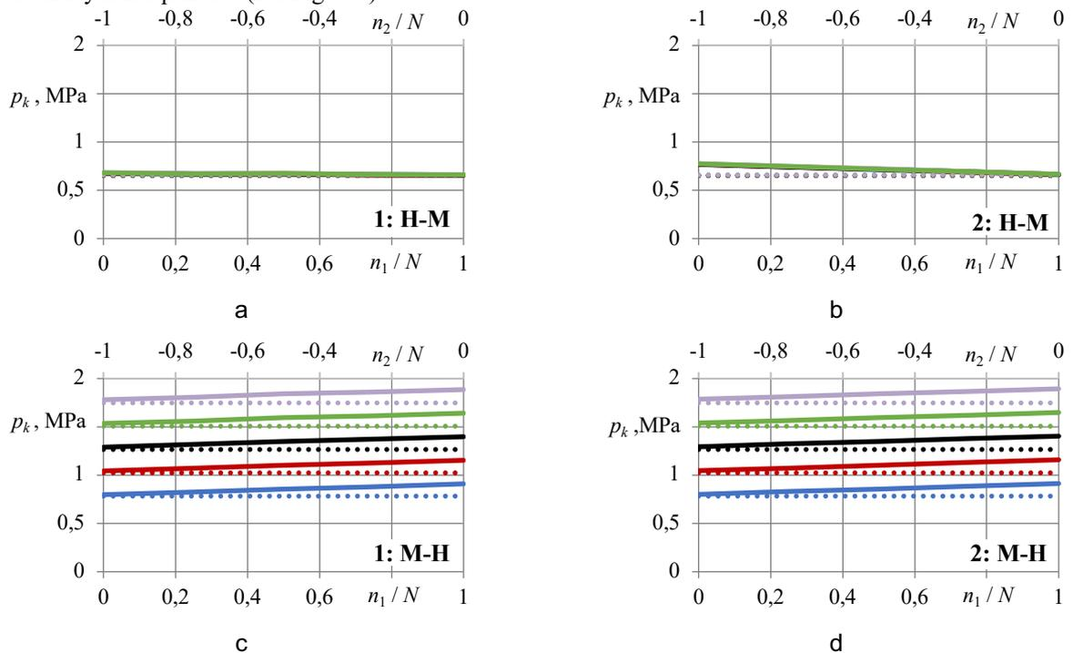
Fig. 7. Dependence of contact pressure  $p_k$  on deviations  $n_1$  and  $n_2$  and internal pressure  $p_0$ , when:  $N = 0.077$  mm;  $d_2 = 14$  mm;  $s_1 = s_2 = 0,5$  mm; ■ –  $p_0 = 0$ ; ■ –  $p_0 = 0,25$  MPa; ■ –  $p_0 = 0,5$  MPa; ■ –  $p_0 = 0,75$  MPa; ■ –  $p_0 = 1$  MPa; a – 1st model H-M type; b – 2nd model H-M type; c – 1st model M-H type; d – 2nd model M-H type; (—) – calculated using BEM; (····) – calculated according to formula
