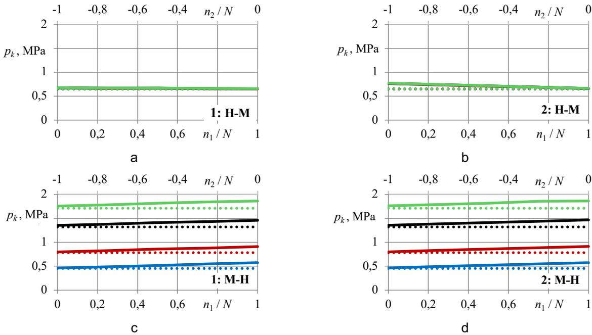
Fig. 5. Dependence of contact pressure  $p_k$  on deviations  $n_1$  and  $n_2$  and inner layer thickness  $s_1$ , when:  $p_0 = 0$ ;  $N = 0,077$  mm;  $d_2 = 14$  mm;  $s_2 = 0,5$  mm; ■ –  $s_1 = 0,3$  mm; ■ –  $s_1 = 0,5$  mm; ■ –  $s_1 = 0,8$  mm; ■ –  $s_1 = 1,0$  mm; a – 1st model H-M type; b – 2nd model H-M type; c – 1st model M-H type; d – 2nd model M-H type; (—) – calculated using BEM; (····) – calculated according to formula (1)
