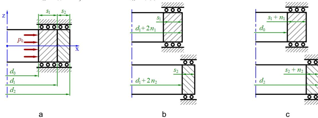
Fig. 1. Flat, axisymmetric model of a two-layer roll: a – calculation scheme; b – model I; c – model II. Here  $n_1$  and  $n_2$  – deviation of the geometry of the inner and outer layers of the roll from the nominal value, respectively
