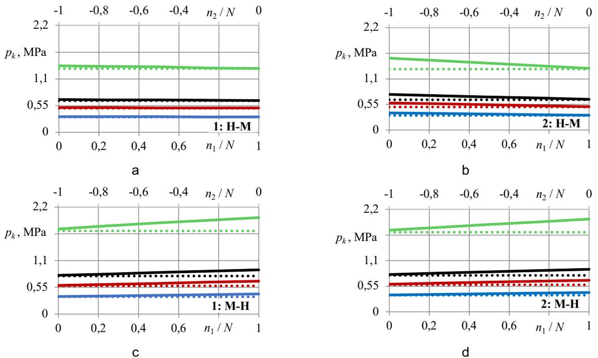
Fig. 4. Dependence of contact pressure  $p_k$  on deviations  $n_1$  and  $n_2$  and outer diameter  $d_2$ , when:  $p_0 = 0$ ;  $N = 0,077$  mm;  $s_1 = s_2 = 0,5$  mm; ■ –  $d_2 = 20$  mm; ■ –  $d_2 = 16$  mm; ■ –  $d_2 = 14$  mm; ■ –  $d_2 = 10$  mm; a – 1st model H-M type; b – 2nd model H-M type; c – 1st model M-H type; d – 2nd model M-H type; (—) – calculated using BEM; (····) – calculated according to formula (1)
