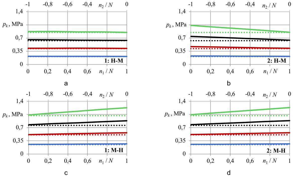
Fig. 3. Dependence of contact pressure  $p_k$  on deviations  $n_1$  and  $n_2$  and stress  $N$ , when:  $p_0 = 0$ ;  $d_2 = 14$  mm,  $s_1 = s_2 = 0.50$  mm; ■ –  $N = 0,025$  mm; ■ –  $N = 0,050$  mm; ■ –  $N = 0,075$  mm; ■ –  $N = 0,100$  mm; a – 1st model H-M type; b – 2nd model H-M type; c – 1st model M-H type; d – 2nd model M-H type; (—) – calculated using BEM; (····) – calculated according to formula (1)
