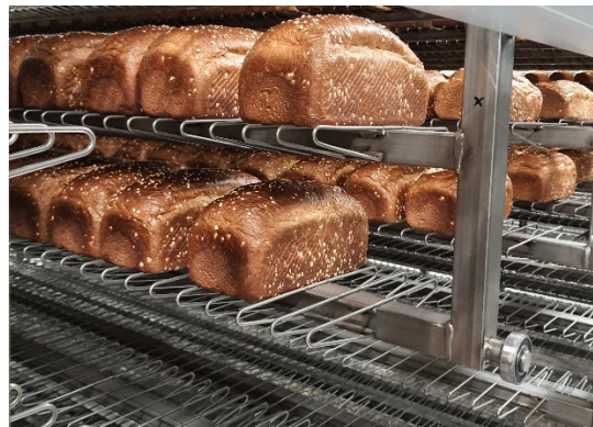
Figure 1. Cooling conveyor hanger with bread
