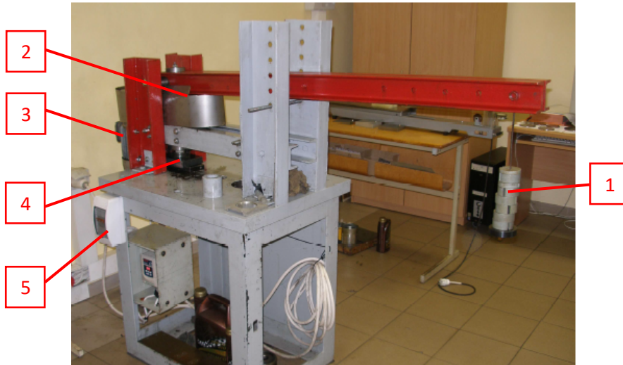
Figure 2. Tribological bearing test stand (1 – load; 2 – the location of the load on the bearing; 3 – engine; 4 – the seat of the bearing under study; 5 – switch with fuses)
