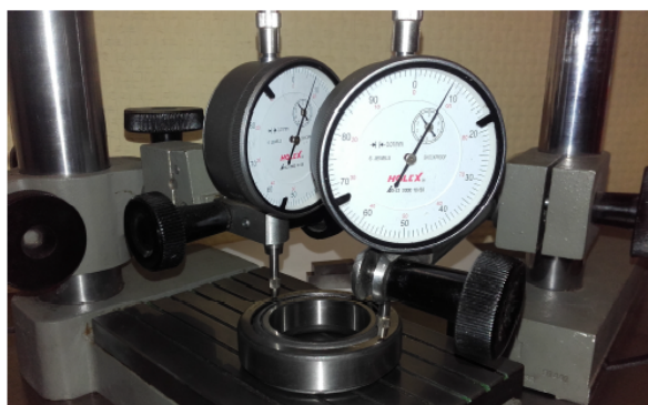
Figure 4. Bearing height change measurements
