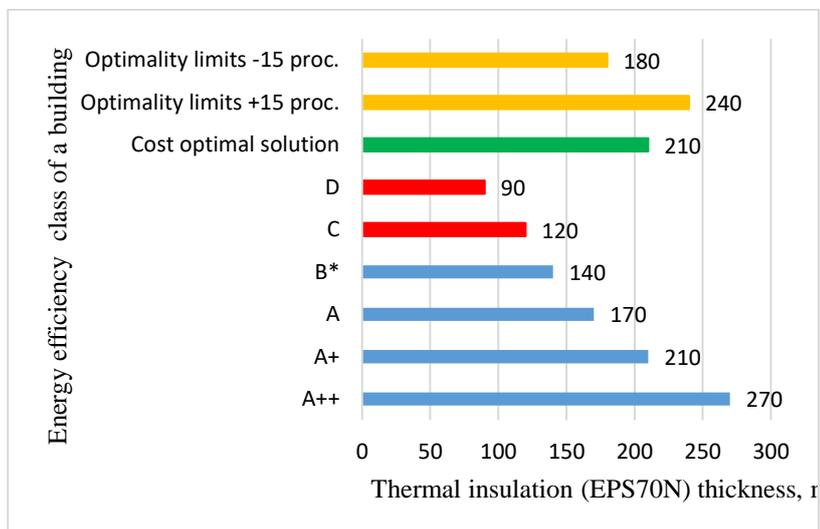
Figure 5. Cost-optimal thermal insulation (EPS70N) thickness for the district heating
