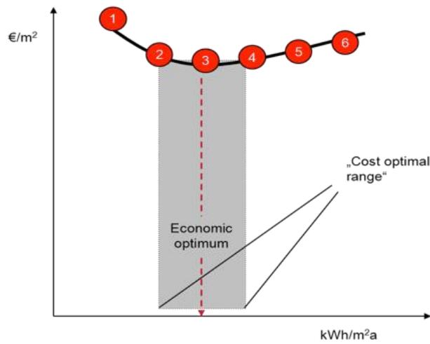
Figure 3. Different variants on the cost-optimal curve and position of the cost-optimal range (BPIE, 2013)
