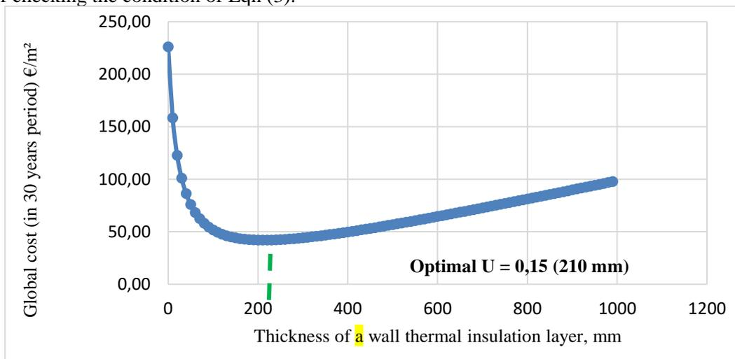
Figure 4. The optimal heat transfer coefficient of the walls of a public building
