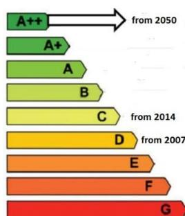
Figure 1. **Min. Requirements for Modernized Buildings (STR 2.01.02:2016)**
