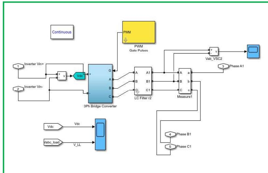
Figure 5. Inverter model with sinusoidal pulse width modulation technique.
