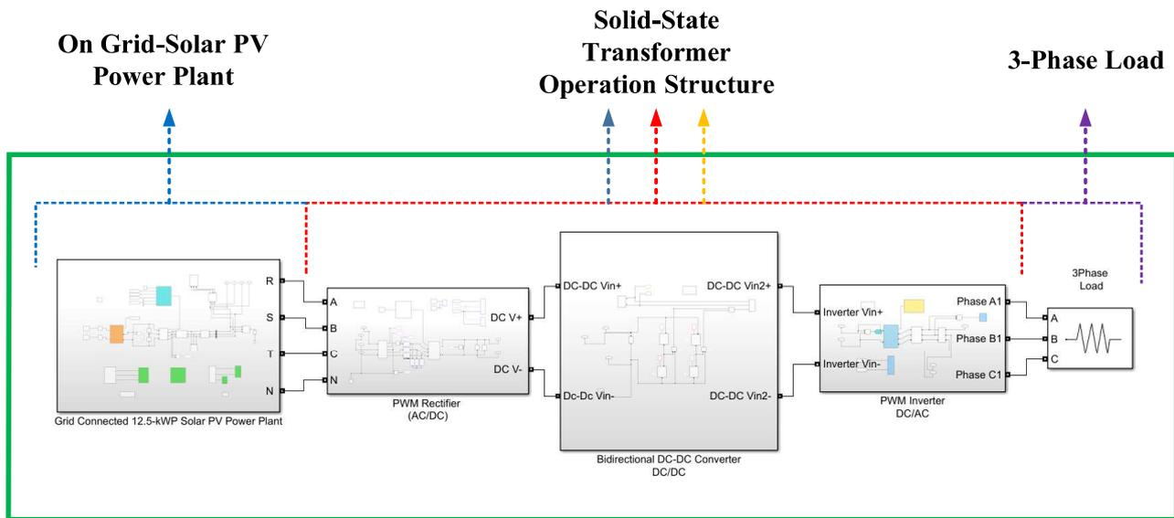
Figure 1. Renewable energy-based three-stage solid-state transformer topology.
