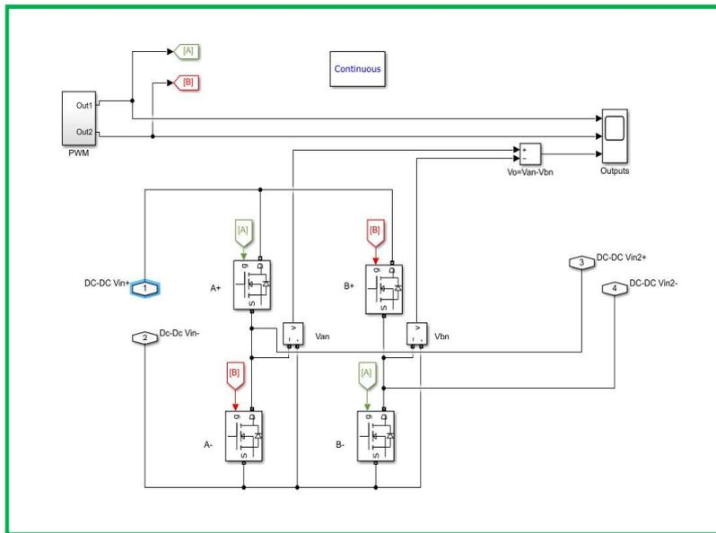
Figure 4. The proposed DC-DC bidirectional converter model.
