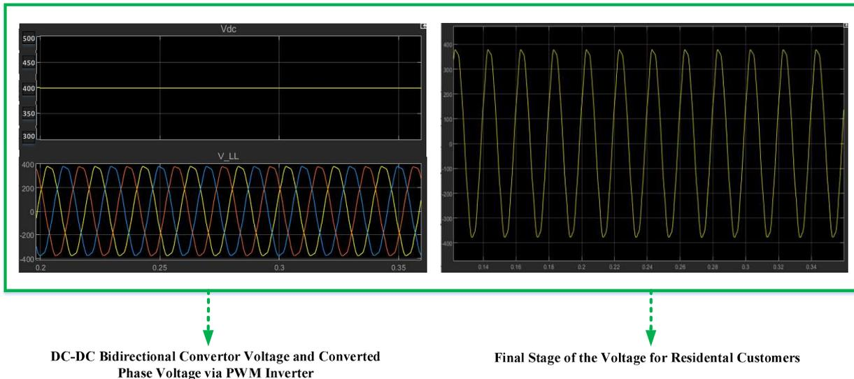
Figure 7. Realization of bidirectional conversion for medium voltage networks and obtaining the desired voltage with PWM inverter.
