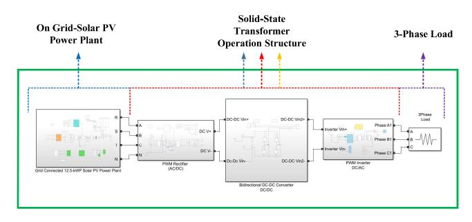
Figure 1. Renewable energy-based three-stage solid-state transformer topology.
