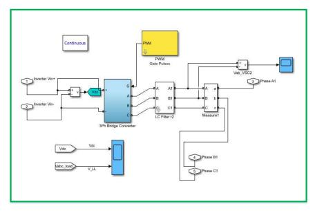
Figure 5. Inverter model with sinusoidal pulse width modulation technique.
