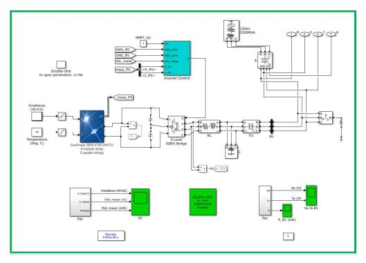
Figure 2. Grid-connected solar power plant controller and its design.
