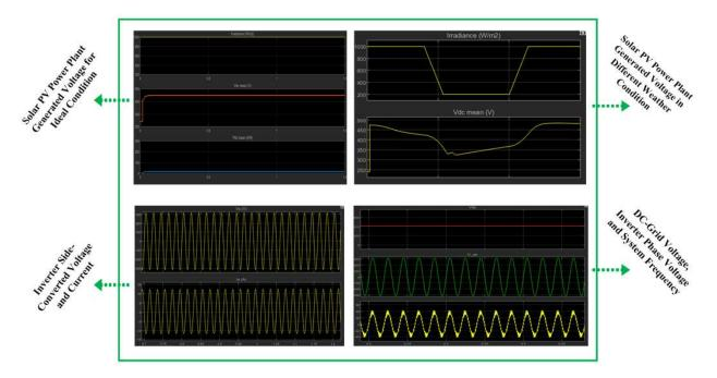
Figure 6. The conversion of voltages generated from the PV plant to alternating current and direct current forms.
