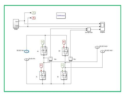
Figure 4. The proposed DC-DC bidirectional converter model.
