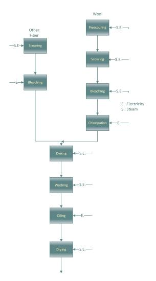
Figure 3. Dyeing and finishing process for fiber and yarn and energy use (Tang & Mohanty, 1996)
